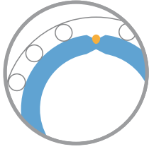
Tack welding of the slit pipe
